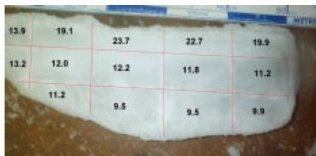
Right: Cross section of pancake 33 showing salinity and portion cut for thin section analysis
