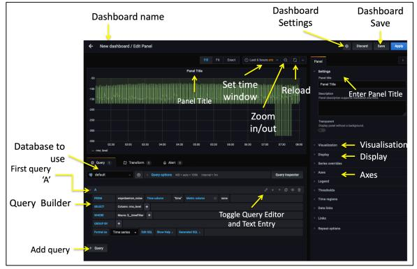
The upper part of the screen shows a default time series graph - a Panel in Grafana jargon. The lower part is a form-filling query builder to collect data from, in our case, a postgreSQL database with TimescaleDB extensions. At right (new in version 7) is an extensive list of option headings to name and then customise the graph. The important Save button is top right - too close to Discard for me!
